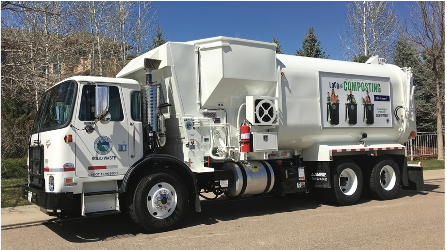
The City of Longmont, Colorado is fueling its collection vehicles with renewable natural gas generated at the city's wastewater treatment plant. Photo courtesy of City of Longmont
